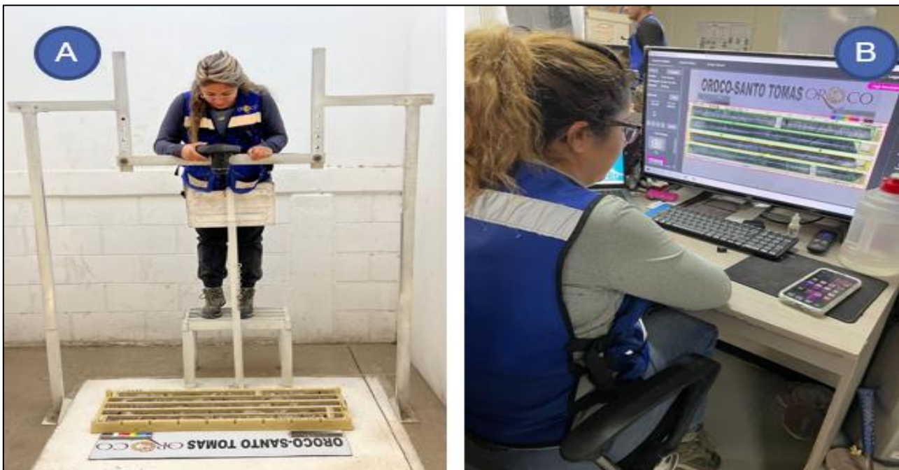
Figure 11-2: A: Core Photo Capture Station at El Ranchito; B: Core Photo Preparation and QA in IMAGO®
