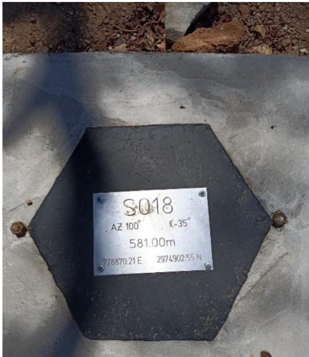
Figure 20-4: Cement Plinth and Metal Label at Drill hole S018, South Zone, Santo Tomás Project
