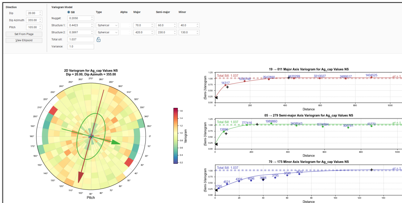
Figure 14-19: Normal Score Transformed Modelled Semi-Variogram for Ag in North Zone Pit
